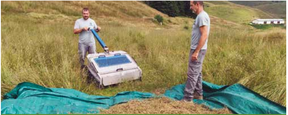
Gathering of brush-harvested seed on a mountain grassland using a special electric motor-powered harvester. The brush-harvested seed is then collected onto a cloth
